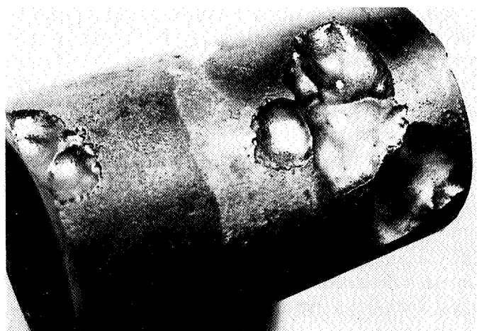
Figure 11. Catastrophic oxidation. Type 316H stainless steel.
